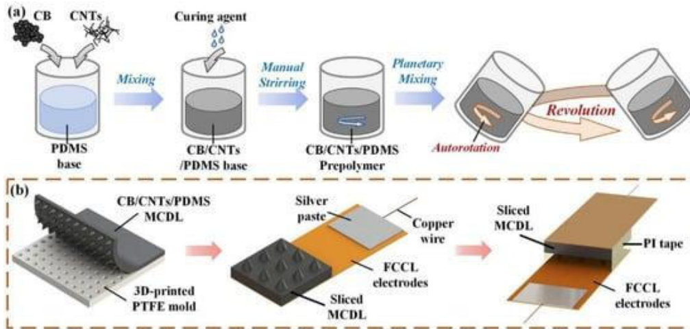
Figure 9.4 Flexible capacitive sensors fabrication [6] pressure sensors based on CB/CNT/PDMS [7]
