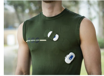
c. Flight Sensing Shirt – Aeolus Physiological monitoring for military pilots [5]
