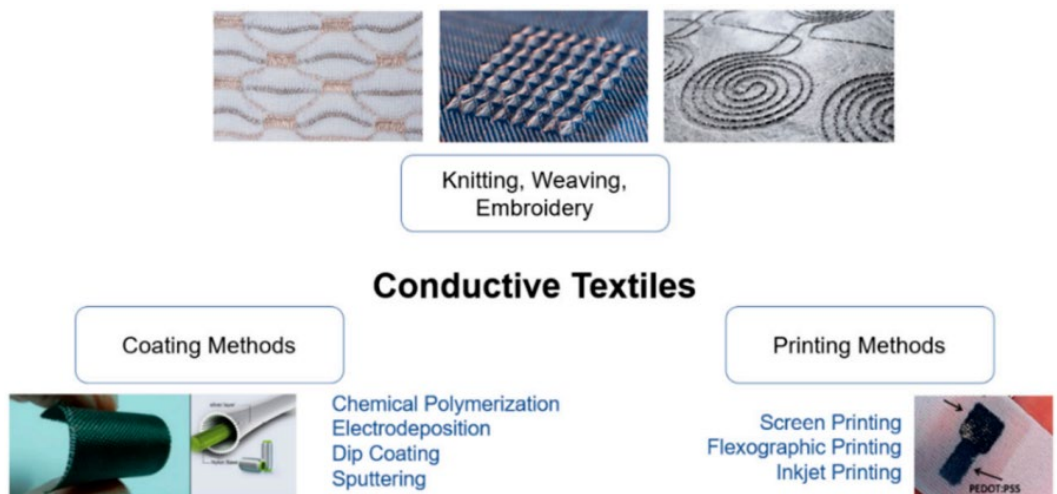
Figure 10.1. Most common manufacturing techniques of conductive textiles: knitting, weaving, embroidery; coating methods; printing [3]
