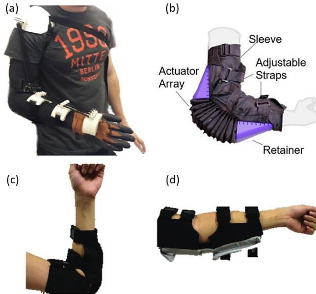
Figure 5.3 (a) A medical rehabilitation exoskeleton for proper patient elbow joint articulation [5]; (b) Design of the soft robotic elbow sleeve [8]; Arm configurations during the use of the soft robotic elbow sleeve. (c) Flexed configuration and (d) Extended configuration [7].
