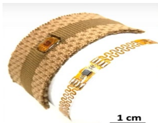
a. Sensors integrated into knit for monitoring temperature, respiration, and heart rate (e-TECS) [7]
