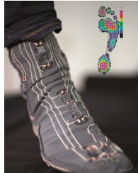
b. Smart sensors for pressure monitoring [4]
