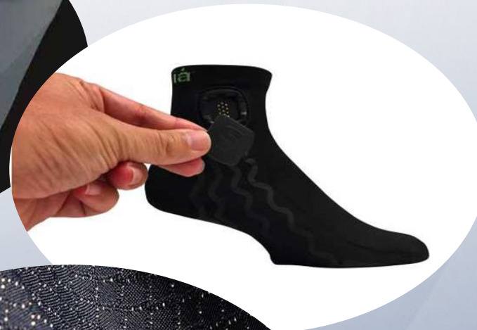
Sensoria Smart Socks: textile sensors detecting parameters important to the running performance
