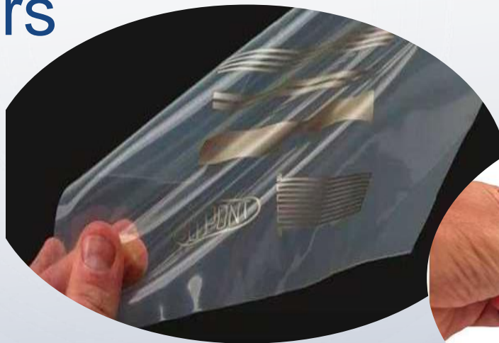
Intexar by DuPont: integration of conductive inks into textiles
